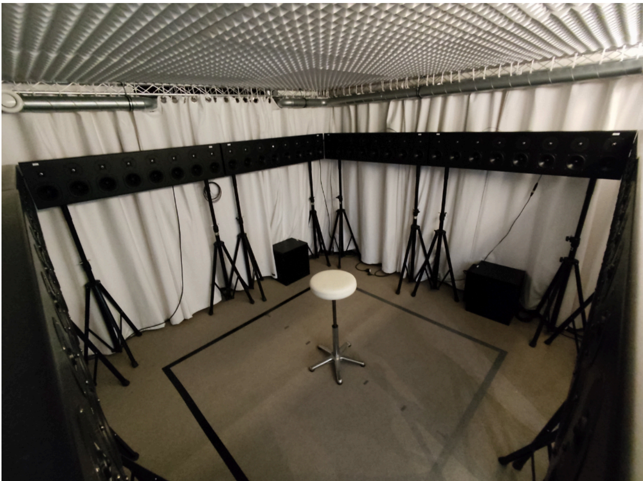
Figure 2: The employed WFS setup at the MPIB. The area marked in black tape corresponds to the WFS-area the participant can move around in.
