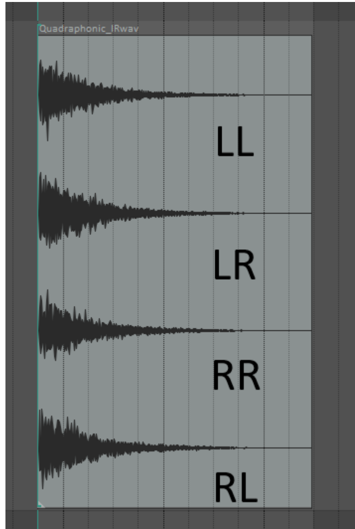
Figure 8: The wave file of the quadrasonic impulse response (IR) corresponding to listening position L2. Each of the four channels is labeled to reflect the channel configuration of a true stereo IR format. The true stereo IR concept will be explained in the next section.
